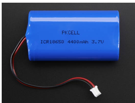
A typical Lithium Ion battery. These usually consist of 1-2 cylindrical cells with pink and blue wrapping.
